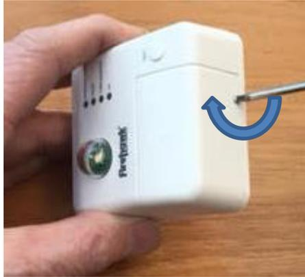
Re-assemble The control Centre to its stand or backplate
